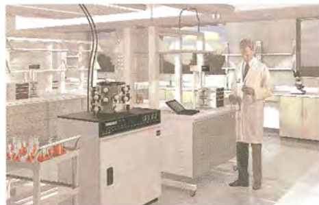
Fig 5. Modular lab and casework design maximizes flexibility to meet project requirements. In these designs, an overhead service carrier and movable casework units enhance the owner's ability to reconfigure lab spaces.
